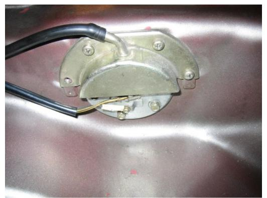
Take the four Phillips head screws off to remove the drain unit. I'm missing one!
