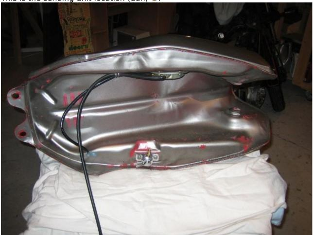
It's the unit on the inside of the tank, with two wires and the drain hose coming from it. There isn't a need to drain all the gas out of the tank, I drained until I hit reserve and left it at that level. Then keep the cap on, and lay it on its side. My Workmate bench is perfect for this as it has two big jaws that open up and can hold the tank nice. Use a blanket so you don't scratch the paint.
